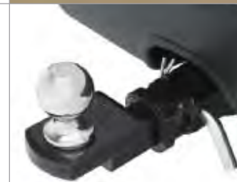
■ Trailer Hitch Subaru hitches are engineered to the same rigorous standards as the rest of your Outback. The hitch is rated at 3,000 lbs. maximum towing capacity with 3.6L engine (2,700 lbs. maximum with 2.5L engine) and 200 lbs. maximum tongue weight. L101SAJ000 Hitch ball not included. Trailer brakes may be needed.
