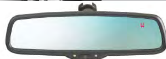
■ Auto-Dimming Mirror with Compass Mirror automatically darkens when headlights are detected from behind the vehicle. Features an electronic compass with a red transfective display that projects the current direction onto the mirror's surface. H501SAJ000
